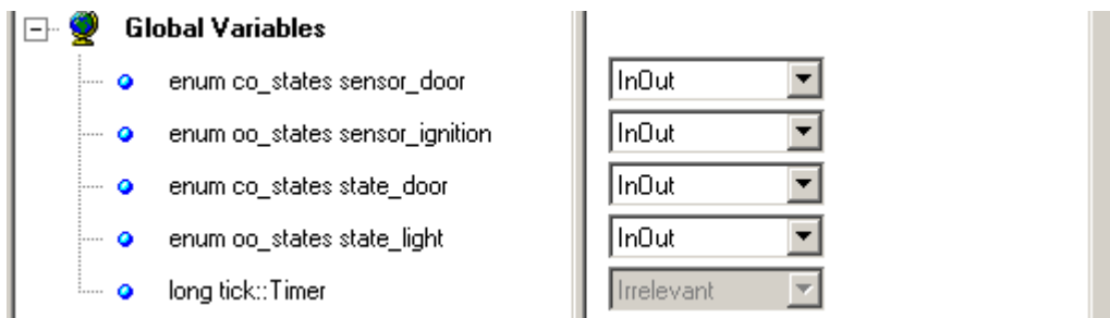
Fig. 20 The initial passing directions of variables used by init()
